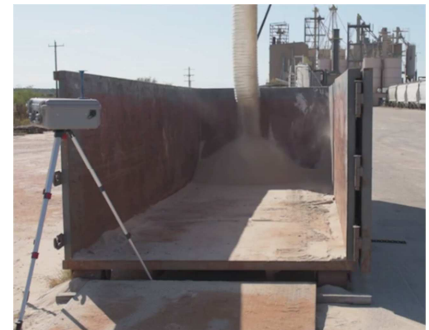
Sentinel Dust Suppressant Treated 100 Mesh Sand Average Respirable Silica: 16 µg/m 3
