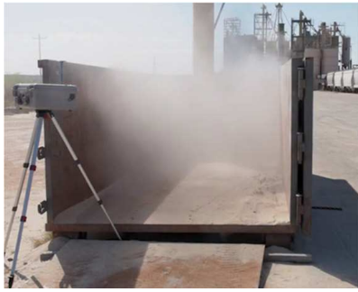
Uncoated 100 Mesh Sand Average Respirable Silica: 1,470 \mu\text{g}/\text{m}^3
