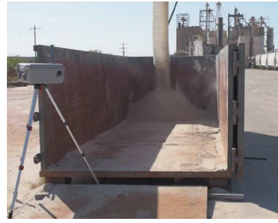
Sentinel Dust Suppressant Treated 100 Mesh Sand Average Respirable Silica: 16 \mu\text{g}/\text{m}^3
